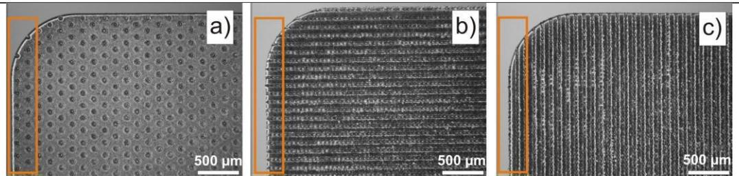
*Surface textures on rake faces of cutting tools (dimple texture (a); channels perpendicular to cutting edge (b) and channels parallel to cutting edge (c))*
